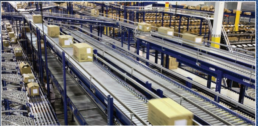
GUESS' WMS automatically directs cartons to their proper destinations and tracks their status in real time.
