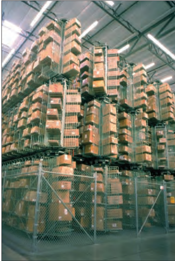
Back view of a three-level horizontal carousel pick area. (Photos courtesy of KardexRemstar)
